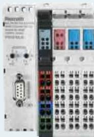
Fieldbus couplers form the first module in an Inline station and are the interface to the fieldbus system. The various I/O modules can be directly connected to these fieldbus couplers.
