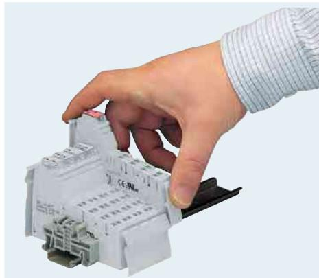
The bus coupler is the head of an Inline station. The I/O modules are simply connected to it end-to-end. All the voltages needed for these modules and the sensors/actuators are automatically cross-wired via the lateral contacts within an Inline station. As a result, all peripheral voltages can be directly tapped.
