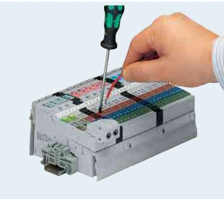
Conductors with stripped ends are simply inserted in the spring-loaded terminals of the Inline connectors without any connector sleeves. Connection cross-sections in the range from 0.2 mm<sup>2</sup> to 1.5 mm<sup>2</sup> are possible.
